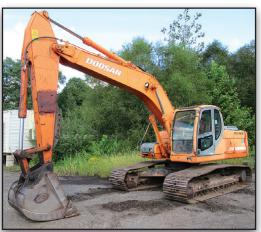
**DOOSAN Model DX225LC Hydraulic** Excavator, s/n 70005038, powered by Doosan diesel engine, equipped with 9'6" dipper stick, Geith 42" digging bucket, thumb bracket, pattern changer, enclosed ROPS cab, and 31.5" TBG pads. In fair to good condition with fair to good undercarriage.
