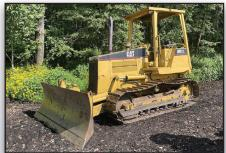
1998 CATERPILLAR Model D4C XL Crawler Tractor, s/n 6YL02137, powered by Cat 3046 diesel engine and powershift transmission, equipped with 6-way straight blade, tow pin, ROPS canopy, and 18" SBG pads. In good condition with good undercarriage. (1,670 Hours on New Undercarriage)
