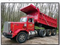
1986 AUTOCAR Tandem Axle **Dump Truck,** powered by Cat 3406B diesel engine and Fuller Roadranger 13 speed transmission, equipped with 14'6" steel dump body with manual tarp, spring/walking beam suspension, Jacobs 3-position engine brake, tow package with air, and 11.00R24 tires. In good condition with good tires. (80,000# GVWR)
