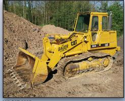
**1997 CATERPILLAR** Model 963B Crawler Loader, s/n 9BL01705, powered by Cat 3116 diesel engine and hydrostatic transmission, equipped with general purpose loader bucket with teeth, enclosed ROPS cab, and 22" DBG pads. In good condition with good to very good undercarriage. (10,419 Hours) (Purchased New)
