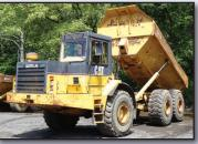
1996 CATERPILLAR Model D350E, 35 Ton, 6x6 Articulated End Dump, s/n 9LR00109, powered by Cat 3406 diesel engine and 4 speed automatic transmission, equipped with lined heatable bed, supplemental steering, enclosed ROPS cab with heat and air conditioning, and 26.5R25 tires. In good condition with fair to good tires.
