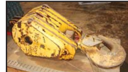
Johnson 100 Ton 5-Sheave Hook Block
