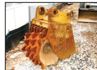
(1) OF (6) COMPACTION WHEELS
