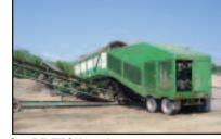
Plant. s/n 1R9TR4724SM216099, powered by John Deere 4045T diesel engine, equipped with 8'x20' feed hopper, 48"x20' incline feed conveyor, 7'x23 screen. 60"x20' trommel discharge under screen conveyor. (2) model 3650R, 36"x50"
