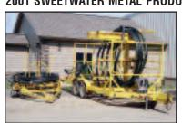
Coiled Pipe Dispensing Trailer. equipped with 8.600# maximum load capacity, McElroy 6,000# line tamer/rerounder/straightener, power adjustable mast, threading rollers, self-loading arm, operators console, and 225/75R15 tires. In good condition with good tires. (Purchased New)
